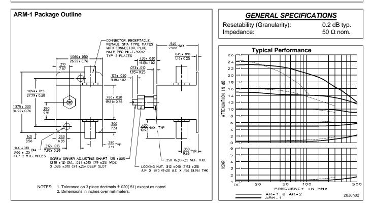
General Note: The AR/ARM series are continuously variable attenuators utilizing compensated Bridged Tee networks to vary signal power. They have the advantage of being very broadband and constant in impedance. Each is designed for high reliability and can be supplied screened to meet specific applications.
