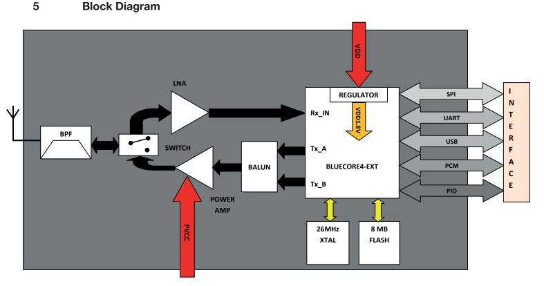
Note: USB and PCM interface are not handled by LM firmware at present
