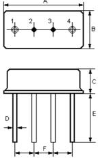
Pin Configuration 1,4 Input / Output 2/3 Case Ground Dimension Data (unit: mm) 11.0±0.3 A В 4.5±0.3 С 3.2±0.3 D 0.45±0.1 Е 5.0±0.5 F 2.54±0.2
