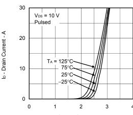
V<sub>GS</sub> - Gate to Source Voltage - V
