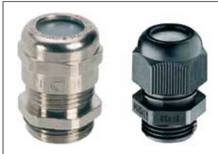
M-EX..PA: - Metric - IP 66 / DIN EN 60529 - Polyamide, black, similar to RAL 9005 - Integrated strain relief - Temperature range : -30°C to +70°C - Test standard: EN 50014/EN50019/ EN50020 - EC test certificates: PTB 99 ATEX 3101 x (M12,M16), PTB 99 ATEX 3128 x (M 20 and higher)
