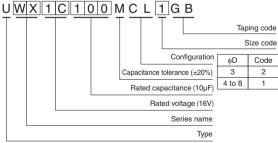
• In the case of size  $\varphi 3$  in ( ),parentheses, use WX in the 2nd and 3rd digit and put a 2 in the 12th digit of type numbering system.
