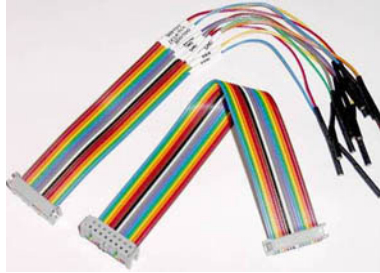
Figure 32 · Ribbon and Breakout Cables
