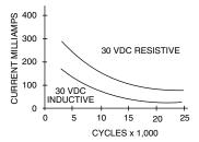
Curve data based on test data conducted at sea level, 25°C and relative humidity. Cycle equals 360° rotation and 360° return. Cycling rate is 10 cycles per minute. The curves shown are typical load life curves for a Series 53M, 57M and 59M Rotary Switch. They show the number of cycles of rotational life that can be expected for the voltages, currents and
