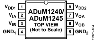
Figure 5. ADuM1240/ADuM1245 8-Lead SOIC (R-8) Pin Configuration
