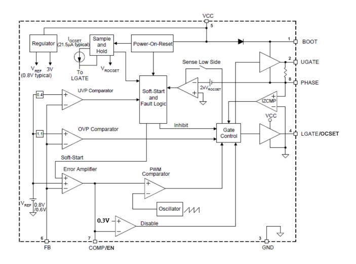
Figure 3. Functional Block Diagram of AP3586A/B/C
