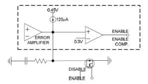
Figure 17. Chip Enable Function
