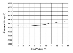
Figure 9. Reference Voltage vs. Input Voltage
