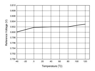
Figure 8. Reference Voltage vs. Temperature
