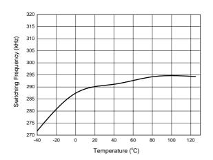
Figure 6. Switching Frequency vs. Temperature
