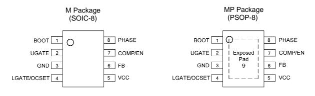
Figure 2. Pin Configuration of AP3586A/B/C (Top View)
