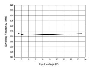
Figure 7. Switching Frequency vs. Input Voltage
