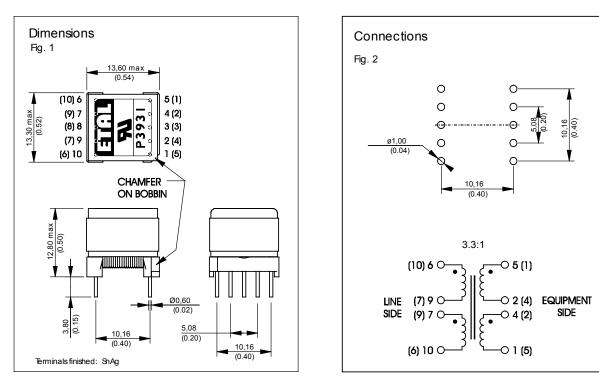
Dimensions shown are in millimetres (inches). Terminal references in parentheses denote alternative customer designation.
