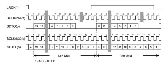
Figure 8. Audio Data Timing (No.1)
