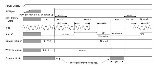
Figure 10. Power-Up / Power-Down Timing Example
