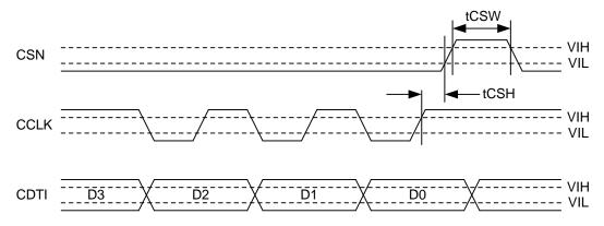
Figure 5. WRITE Data Input Timing
