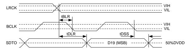
Figure 3. Audio Data Output Timing (Audio I/F = No.0)
