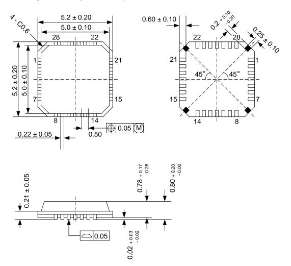
Note) The part of black at four corners on reverse side must not be soldered and must be open.
