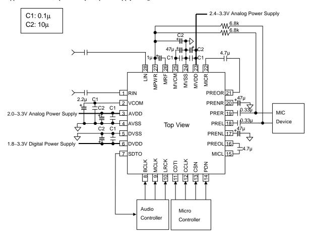
Figure 13. System Connection Diagram Example
