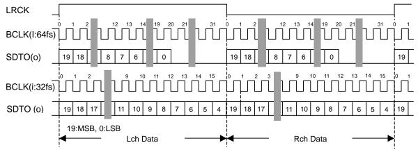
Figure 7. Audio Data Timing (No.0)
