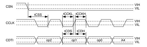
Figure 4. WRITE Command Input Timing
