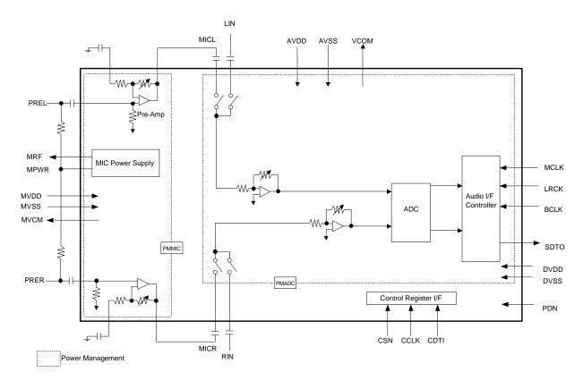
Figure 1. AK5356 Block Diagram
