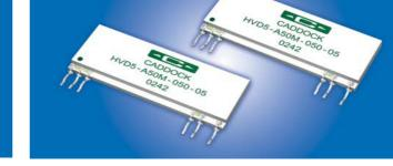
**Type HVD Ultra-Precision Voltage Dividers** are monolithic voltage dividers built with ceramic sandwich construction. These voltage dividers have ultra-precision performance in the range of 1500 volts DC to 5000 volts DC, with a Ratio Tolerance of 0.05% and Ratio TC of 5ppm/°C. These dividers are ideal for high performance voltage division applications in medical equipment, laboratory equipment, analytical instruments, etc.
