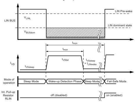
Figure 2-4. Short-circuit to GND on the LIN Bus During Sleep Mode
