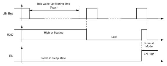
In Sleep mode the device has a very low current consumption even during short-circuits or floating conditions on the bus. A floating bus can arise if the master pull-up resistor is missing, e.g., it is switched off when the LIN master is in sleep mode or even if the power supply of the master node is switched off.
