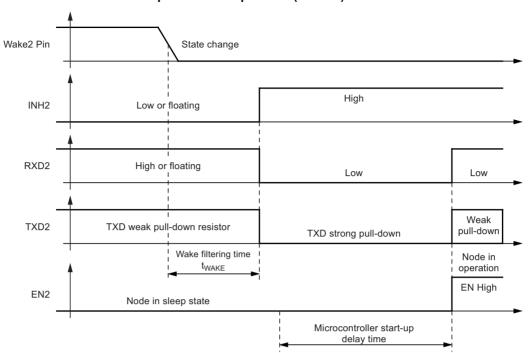
Figure 2-5. LIN Transceiver 2: Wake-up from Wake-up Switch (WAKE2)
