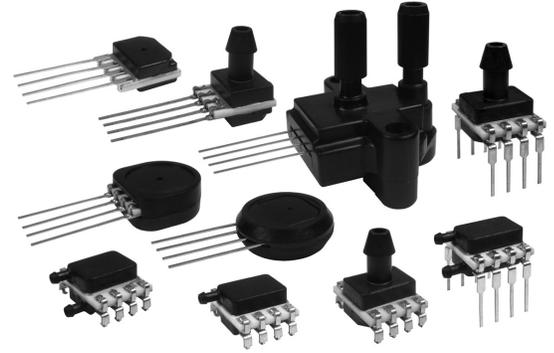
**The pressure is on. The answer is here.** No matter the need, Honeywell Sensing and Control (S&C) has the microstructure, pressure sensor solution. Our sensing element design consists of four piezoresistors on a chemically etched silicon diaphragm. A pressure change will cause a strain in the diaphragm and the buried resistors. The resistor values will change in proportion to the stress applied, which produces an electrical output. You
