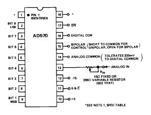
Figure 4. Standard AD570 Connections
