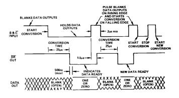
Figure 9. AD570 Timing and Control Sequence
