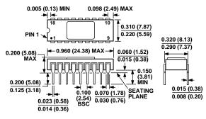
CONTROLLING DIMENSIONS ARE IN INCHES; MILLIMETER DIMENSIONS (IN PARENTHESES) ARE ROUNDED-OFF INCH EQUIVALENTS FOR REFERENCE ONLY AND ARE NOT APPROPRIATE FOR USE IN DESIGN.
