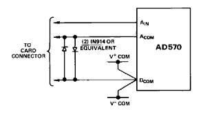
Figure 6. Differential Common Voltage Protection
