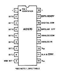
Figure 3. AD570 Pin Connections
