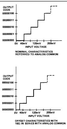
Figure 8. AD570 Transfer Curve—Unipolar Operation (Approximate Bit Weights Shown for Illustration, Nominal Bit Weights ~ 36.1 mV)
