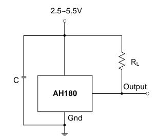
Note: C is for power stabilization and to strengthen the noise immunity, the recommended capacitance is 10nF~100nF. R<sub>L</sub> is the pull-up resistor, the recommended resistance is 10Kohm~100Kohm.
