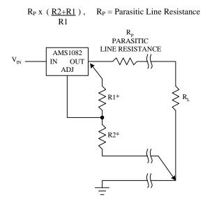
Connected as shown, R<sub>P</sub> is not multiplied by the divider ratio. Using 16-gauge wire the parasitic line resistance is about 0.004 $\Omega$  per foot, translating to 4mV/ft at 1A load current. It is important to keep the positive lead between regulator and load as short as possible and use large wire or PC board traces.
