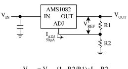
$V_{OUT} = V_{REF} (1 + R2/R1) + I_{ADJ}R2$
