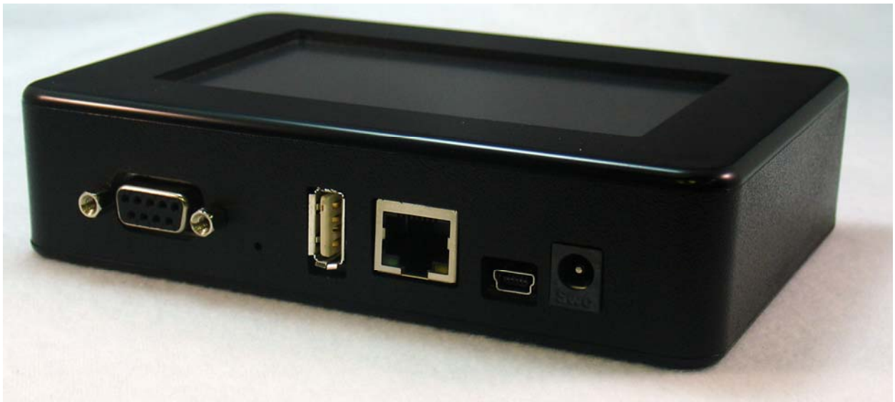
uEZGUI-2478-43WQS with uEZGUI-EXP1 mounted in OEM Housing
