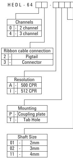
\* 4mm shaft size is not available for 3 channel devices.
