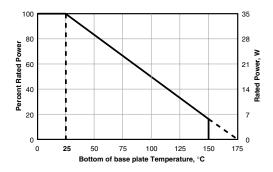
Derating (thermal resistance): 0.23W/°C (4.28°C/W). The case temperature is to be used for purposes of establishing the applied power limit. The case temperature measurement must be made with a thermocouple contacting the center of the component mounted on the designed heat sink. Thermal grease should be applied propperly.
