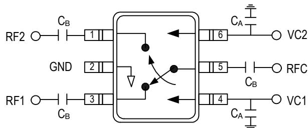
DC blocking capacitors  $C_B$  are required on all RF ports.  $C_B = C_A = 51\text{pF}$  for operating frequency > 500MHz.
