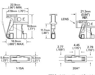
\*20A Fuseholder must be used. Fuse is keyed to prevent insertion in lower rated holders. 20A Fuseholder is designed to accept all ratings up to 20 amperes.
