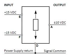
A through F: Connector pin assignments
