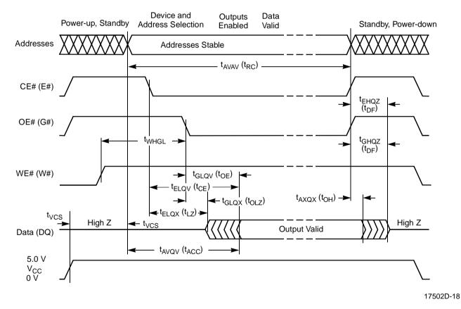
Figure 9. AC Waveforms for Read Operations
