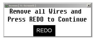
This screen appears after **REDO** has been pressed on either Screen 6 or 7. When all the wires have been removed, press **REDO** to return to Screen 6 or 7.
