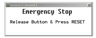
This screen is displayed when the Emergency Stop button has pressed. It also appears after power up and after the Safety Guard Open screen, when the door has been closed. Release the Emergency Stop button and press the blue reset button on the main Panel.
