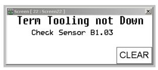
This screen is displayed when the Termination Tooling Cylinder fails to activate sensor B1.03 (See Section 2.2.6).. Check to see if the tooling jammed or if something is stopping the cylinder from completing its stroke. Clear the fault and press **CLEAR** button.
