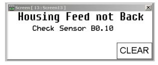
This screen is displayed when the Housing Feed Cylinder (See Section 2.2.2) fails to activate sensor B0.10. Check to see if the tooling jammed or if something is stopping the cylinder from completing its stroke. Clear the fault and press **CLEAR** button.
