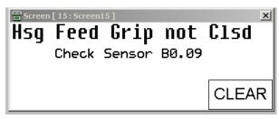
This screen is displayed when the Housing Feed Gripper Cylinder (See Section 2.2.1) fails to activate sensor B0.09. Check to see if the tooling jammed or if something is stopping the cylinder from completing its stroke. Clear the fault and press **CLEAR** button.
