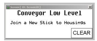
This screen is displayed when the connector conveyor level is low. Join another chain to the existing chain and press the **CLEAR** button to continue
