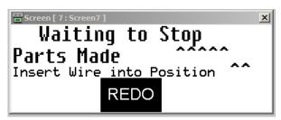
This screen is displayed after the stop button has been pressed and before the current cycle has been completed.
