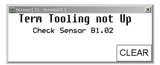
This screen is displayed when the Termination Tooling Cylinder fails to activate sensor B1.02, (See Section 2.2.6). Check to see if the tooling jammed or if something is stopping the cylinder from completing its stroke. Clear the fault and press **CLEAR** button.
