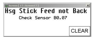
This screen is displayed when the Housing Stick Feed Cylinder fails to activate sensor B0.07. Check to see if the tooling jammed or if something is stopping the cylinder from completing its stroke. Clear the fault and press **CLEAR** button.
