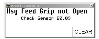
This screen is displayed when the Housing Feed Gripper Cylinder(See Section 2.2.1) fails to deactivate sensor B0.09. Check to see if the tooling jammed or if something is stopping the cylinder from completing its stroke. Clear the fault and press **CLEAR** button.
