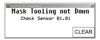
This screen is displayed when the Mask Tooling Cylinder (See Section 2.2.4) fails to activate sensor B1.01. Check to see if the tooling jammed or if something is stopping the cylinder from completing its stroke. Clear the fault and press **CLEAR** button.
