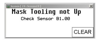
This screen is displayed when the Mask Tooling Cylinder (See Section 2.2.4) fails to activate sensor B1.00. Check to see if the tooling jammed or if something is stopping the cylinder from completing its stroke. Clear the fault and press **CLEAR** button.
