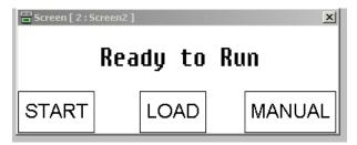
This screen is displayed when the machine is stopped and there are no fault conditions. It has 3 buttons located on the bottom.
