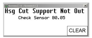
This screen is displayed when the Housing Cut Support Cylinder (See Section 2.2.2) fails to activate sensor B0.05. Check to see if the tooling jammed or if something is stopping the cylinder from completing its stroke. Clear the fault and press **CLEAR** button.
