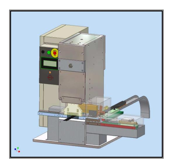
RAST 2.5 Power SEMI-AUTOMATIC TERMINATOR MACHINE
