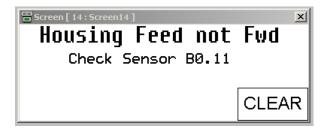
This screen is displayed when the Housing Feed Cylinder (See Section 2.2.2) fails to activate sensor B0.11. Check to see if the tooling jammed or if something is stopping the cylinder from completing its stroke. Clear the fault and press **CLEAR** button.
