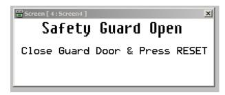
This screen is displayed when the safety guard is open. Close the guard and press the blue reset button on the main panel.
