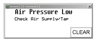
This screen is displayed when the Air Pressure coming to the Machine is Low. Air pressure less than approx. 4 bar / 60 psi. Check the following:
