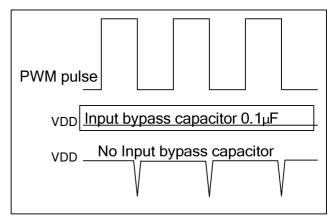
Figure 3. Input Bypass Capacitor Affects the  $V_{\text{DD}}$  Drop.
