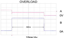
A: V<sub>OUT1</sub>,5 V/ div B: INDUCTOR CURRENT,1A/ div
