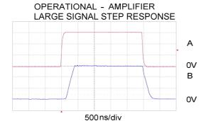
A: INPUT SIGNAL,2V/div B: OUTPUT SINAL,2V/div V<sub>SUP</sub>= 6V
