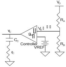
Figure 6. Voltage Loop Compensator
