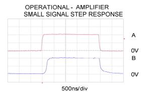
A: INPUT SIGNAL, 200 mV/div B: OUTPUT SINAL, 200 mV/div
