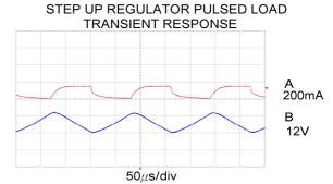
A: LOAD CURRENT,100mA/div B: V<sub>OUT1</sub>, 200mV/div, AC-COUPLED
