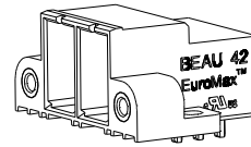
2 AND 3 CIRCUIT HEADERS HAVE NO "PRY SLOTS"
