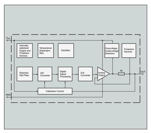
Fig. 1: Block diagram of the HAL 1821/1822/1823
