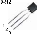
1.Gate 2. Drain 3. Source
