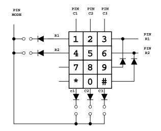
Double contacts under keys 0-9\*#: One contact is connected to AS2540, the other one to CPU.
