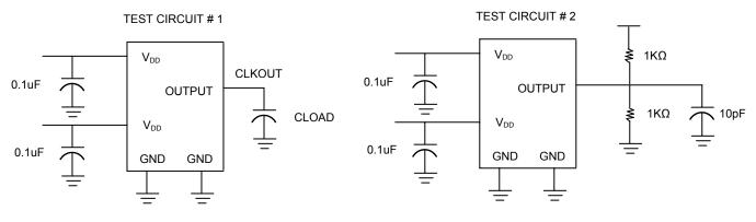
For parameter  $t_{8}$  (output skew rate) on -1H devices
