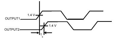
Input - Output Propagation Delay
