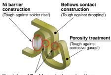
V notch and Double contact constructions
