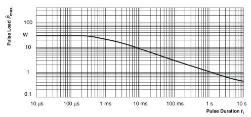
Maximum pulse load, single pulse; applicable if  $\bar{P} \rightarrow 0$  and  $n \le 1000$  and  $\hat{U} \le \hat{U}_{max}$ ; for permissible resistance change equivalent to 8000 h operation Single Pulse
