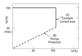
Typical LED power supply I-V curve
