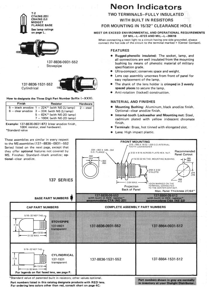
Order complete with lamp to be assured of receiving the indicator light and correct lamp together for immediate use.
