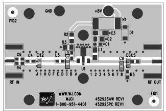
Circuit Board Material:  $.014^{\circ}$  Getek, 4 - layer, 1 oz copper, Microstrip line details: width =  $.026^{\circ}$ , spacing =  $.026^{\circ}$ . The silk screen markers 'A', 'B', 'C', etc. and '1', '2', '3', etc. are used as placemarkers for the input and output tuning shunt capacitors. The markers and vias are spaced in  $.050^{\circ}$  increments. C7/C8 are for 900 MHz matching circuits and C9/C12 are for 1900 MHz matching circuits.
