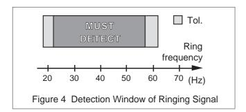
When a continious valid ring signal is present for 80 ms, the melody generator is activated and remains active until two or more periods of the ring signal are missing.
