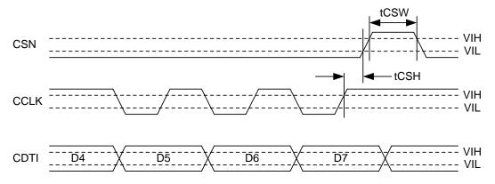
Figure 4. WRITE Data Input Timing
