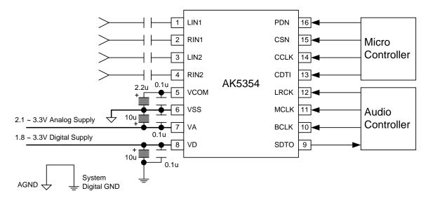
Figure 12. System Connection Diagram Example
