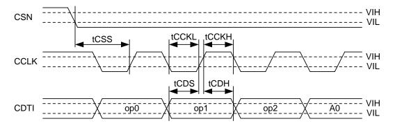
Figure 3. WRITE Command Input Timing
