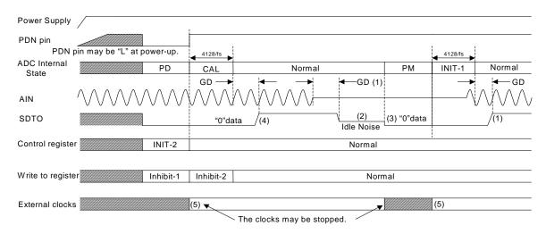
Figure 8. Power up / Power down Timing Example
