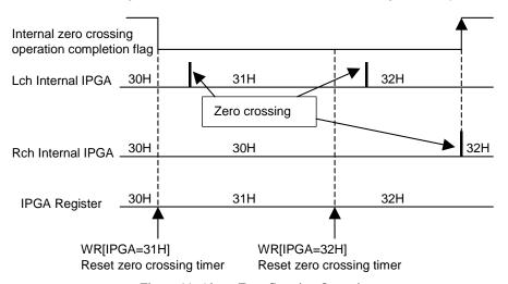
Figure 11. About Zero Crossing Operation
