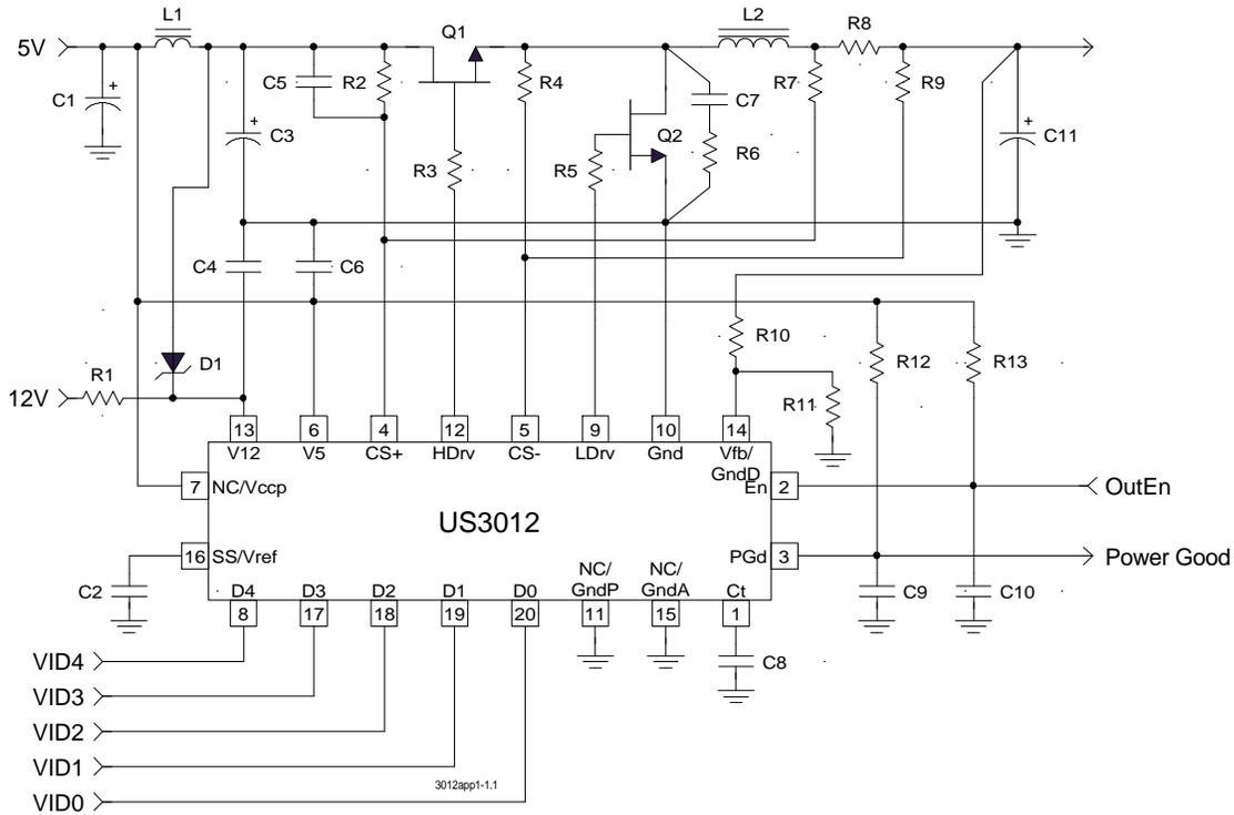
Typical application of US3012/3012A in an on board DC-DC converter providing the Core supply for the Pentium II microprocessor.
