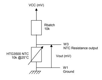
$$V_{OUT}(mV) = \frac{Vcc(mV) * NTC_{HTG3500}(\Omega)}{R_{batch}(\Omega) + NTC_{HTG3500}(\Omega)}$$
