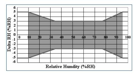
HTG3500 series modules are specified for maximum accuracy measurements within 10 to 95 %RH.
