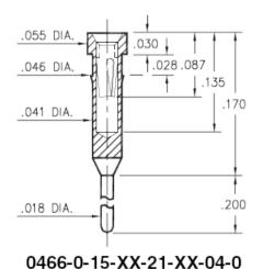
Press-fit in .043 mounting hole. shell is Phos. Br. Alloy 544 (B2)
