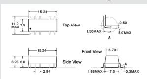
Note: All Pins on a 2.54mm pitch; All Pin diameters are 0.50 mm (Tolerance: $\pm 0.25$ ); All dimensions in mm.
