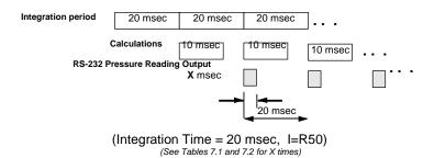
Figure 7.5—Timing Diagram for 50 Readings Per Second
