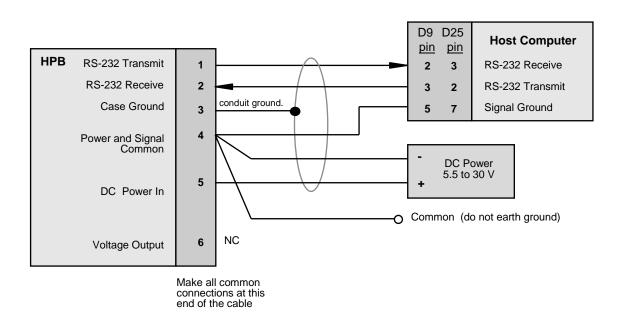
Figure 6.2—Connection for RS-232 Operation
