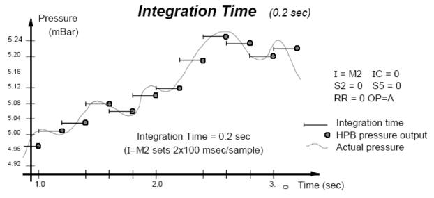
Figure 4.5—Integration (I=) Command, Example 1
