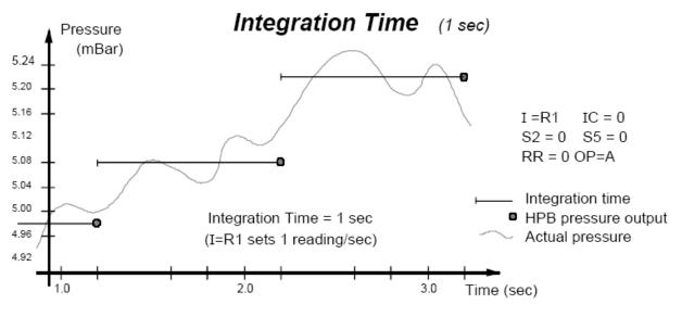
Figure 4.6—Integration (I=) Command, Example 2
