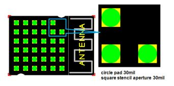
Figure 9: Solder Stencil Reference
