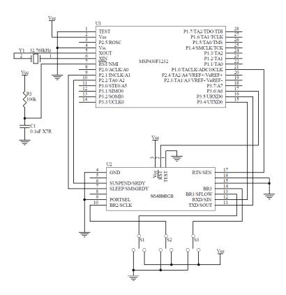
Figure 14: N548M8CB ANT NP Configuration Connection
