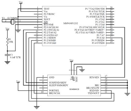
Figure 15: N548M4CB ANT NP Configuration Byte Sync Connection
