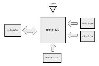
Figure 3: N5 ANT SoC Module Series Block Diagram
