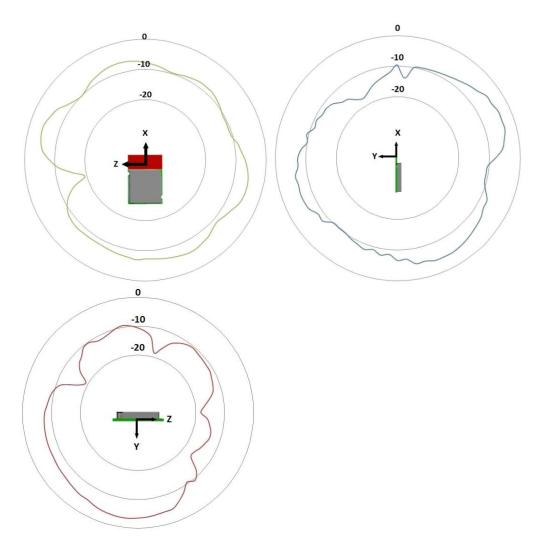
Table 8: N5 M4 Module Typical Antenna Gain (dBi)
