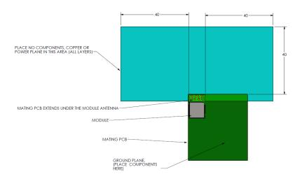
Figure 7: N5 M8 Module Mounting (all dimensions in mm)
