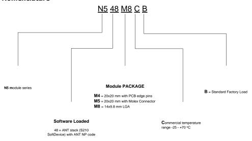
Figure 1: N5 ANT SoC Module Series Nomenclature
