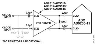
Figure 26. Differential LVDS Sample Clock
