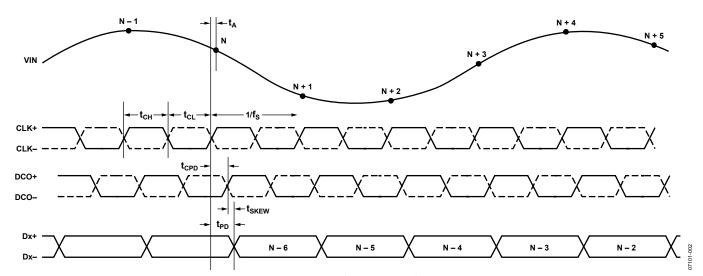
Figure 2. Single Data Rate Mode
