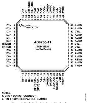
Figure 4. Single Data Rate Mode Pin Configuration
