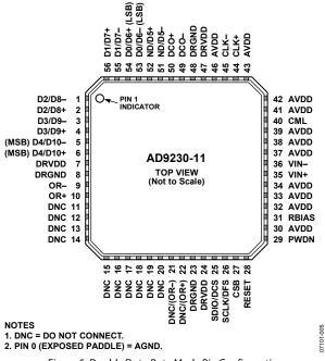
Figure 5. Double Data Rate Mode Pin Configuration
