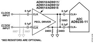
Figure 25. Differential PECL Sample Clock
