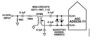
Figure 24. Transformer-Coupled Differential Clock
