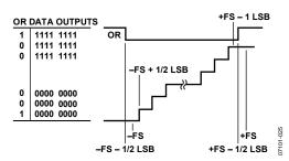
Figure 32. OR Relation to Input Voltage and Output Data
