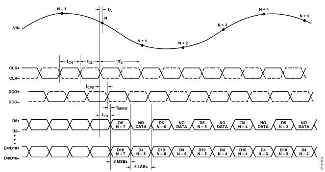
Figure 3. Double Data Rate Mode
