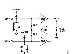
Figure 16. Analog Inputs ( $V_{CML} = \sim 1.4 \text{ V}$ )
