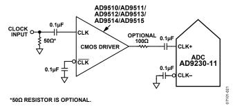
Figure 28. Single-Ended 3.3 V CMOS Sample Clock
