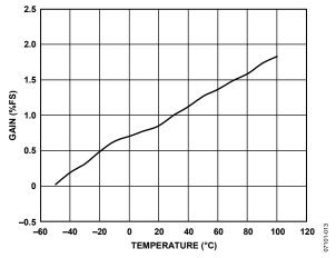
Figure 13. Gain vs. Temperature
