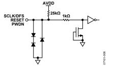
Figure 17. Equivalent SCLK/DFS, RESET, PWDN Input Circuit
