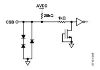
Figure 18. Equivalent CSB Input Circuit
