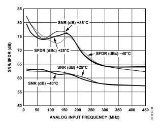
Figure 9. Single-Tone SNR/SFDR vs. Input Frequency (f<sub>IN</sub>) with 1.25 V p-p Full-Scale; 200 MSPS
