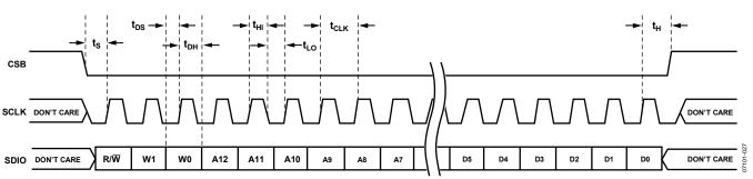
Figure 33. Serial Port Interface Timing Diagram
