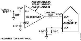
Figure 27. Single-Ended 1.8 V CMOS Sample Clock
