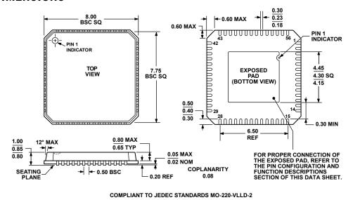
Figure 34. 56-Lead Lead Frame Chip Scale Package [LFCSP\_VQ] 8 mm × 8 mm Body, Very Thin Quad (CP-56-2)
