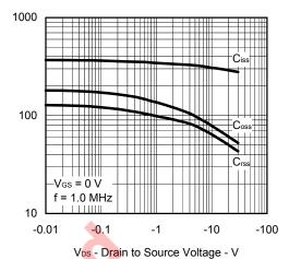
CAPACITANCE vs. DRAIN TO SOURCE VOLTAGE
