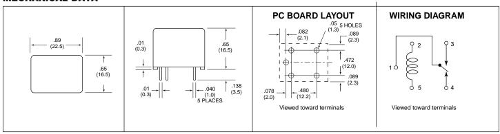
Dimensions in inches with metric equivalents in parentheses. Tolerance: ±0.010"
