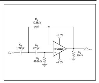
Figure 9. 10kHz High-Pass Filter
