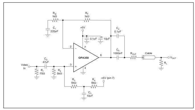
Figure 6. Single-Supply Video Line Driver
