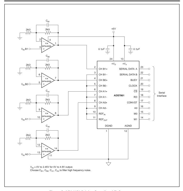
Figure 5. OPA4350 Driving Sampling A/D Converter
