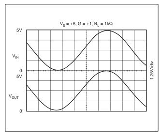
Figure 1. Rail-to-Rail Input and Output
