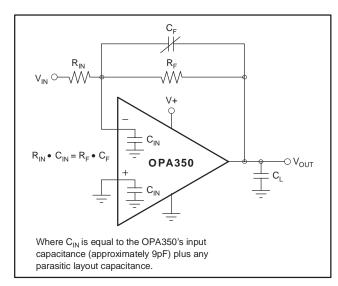
Figure 4. Feedback Capacitor Improves Dynamic Performance
