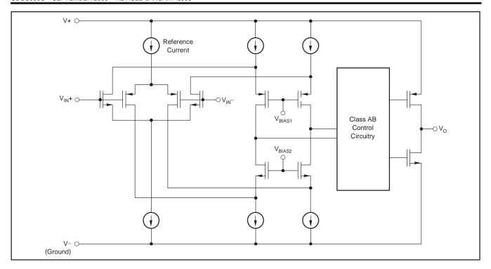
Figure 2. Simplified Schematic
