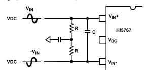
FIGURE 17. DC COUPLED DIFFERENTIAL INPUT
