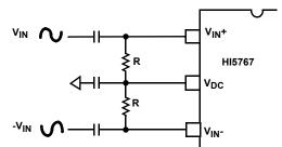
FIGURE 16. AC COUPLED DIFFERENTIAL INPUT
