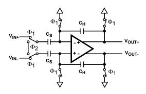
FIGURE 15. ANALOG INPUT SAMPLE-AND-HOLD
