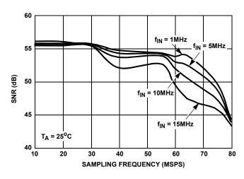
FIGURE 3. SNR vs SAMPLING FREQUENCY
