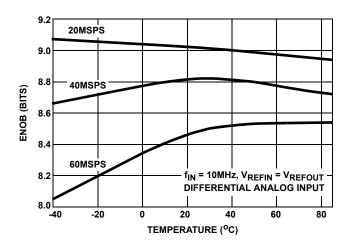
FIGURE 9. EFFECTIVE NUMBER OF BITS (ENOB) vs TEMPERATURE
