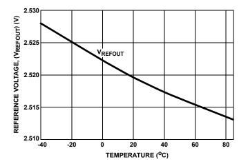
FIGURE 10. INTERNAL REFERENCE VOLTAGE ( $V_{REFOUT}$ ) vs TEMPERATURE
