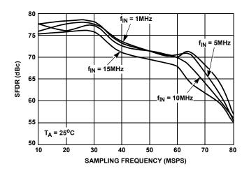
FIGURE 5. SFDR vs SAMPLING FREQUENCY
