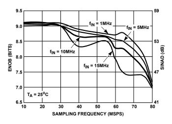
FIGURE 2. EFFECTIVE NUMBER OF BITS (ENOB) AND SINAD vs SAMPLING FREQUENCY
