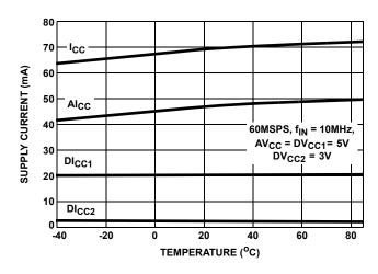
FIGURE 13. SUPPLY CURRENT vs TEMPERATURE
