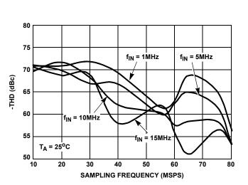
FIGURE 4. -THD vs SAMPLING FREQUENCY
