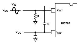
FIGURE 19. DC COUPLED SINGLE ENDED INPUT
