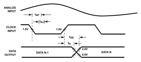
FIGURE 1. INPUT TO OUTPUT TIMING
